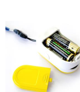
Figure 3. Installation des piles
